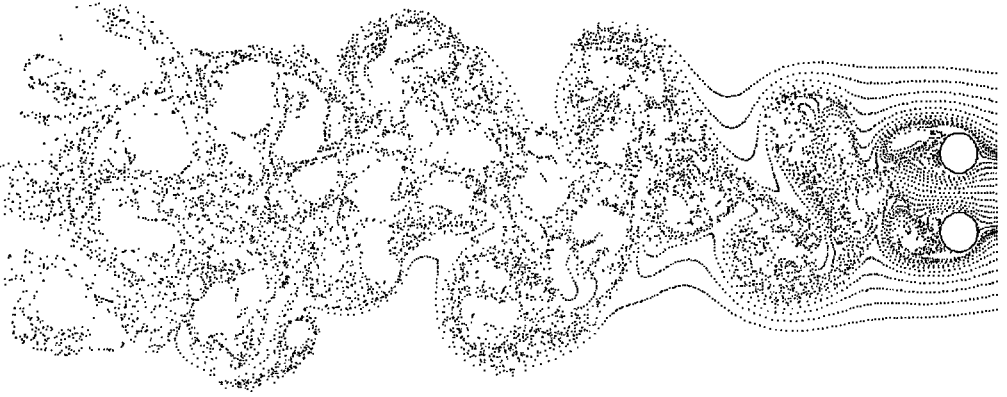
Figure 2: Streaklines about two cylinders, g^* = 1 .
