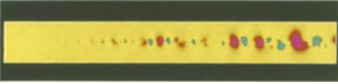
Fig. 2. V-velocity Gouraud shaded contours at 12,000 timesteps. The step function is used as a initial condition.
