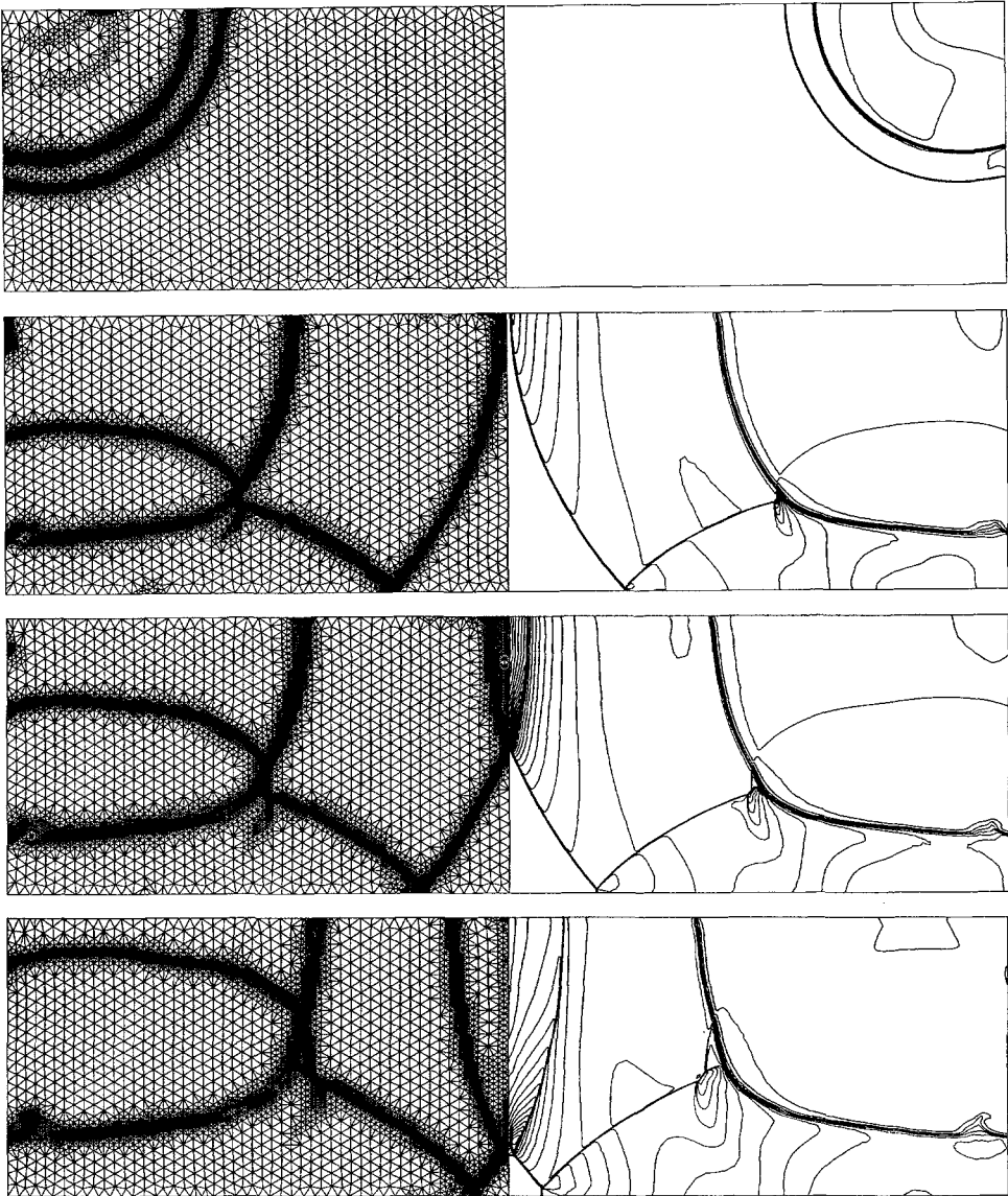
Figure 3. The time history of a toroidal shock wave interaction with the symmetry axis and wall (density contour lines and the respective grids)
