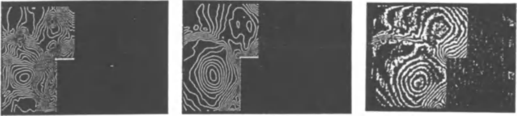
Figure 4: Comparison of the density contours inside a rectangular piston-engine model with a step-piston for several intake strokes at 90^\circ CA (left: first stroke, center: second stroke, right: experiment)
