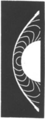
Fig. 3 Euler solution for circular cylinder; M = 10 , 61 \times 61 grid.
