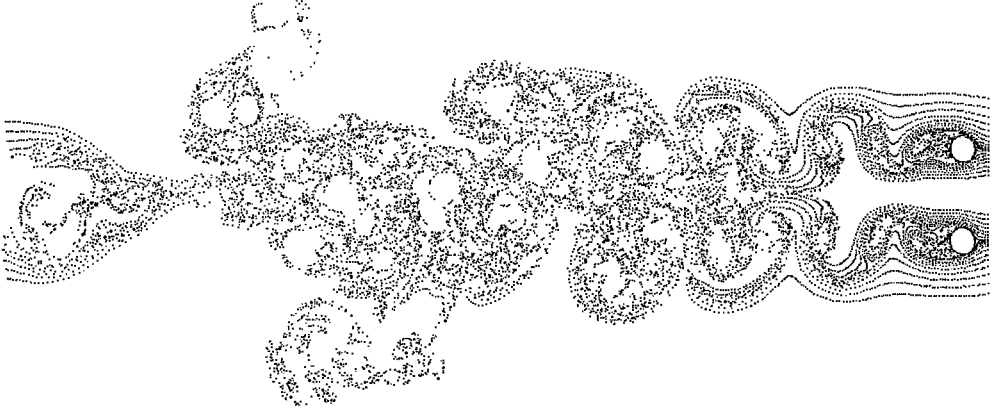
Figure 1: Streaklines about two cylinders, g^* = 2.5 .
